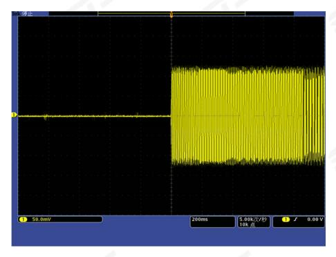
Transmitter Frequency Behaviour @ 12.5 KHz Channel Separation-----On - Off
