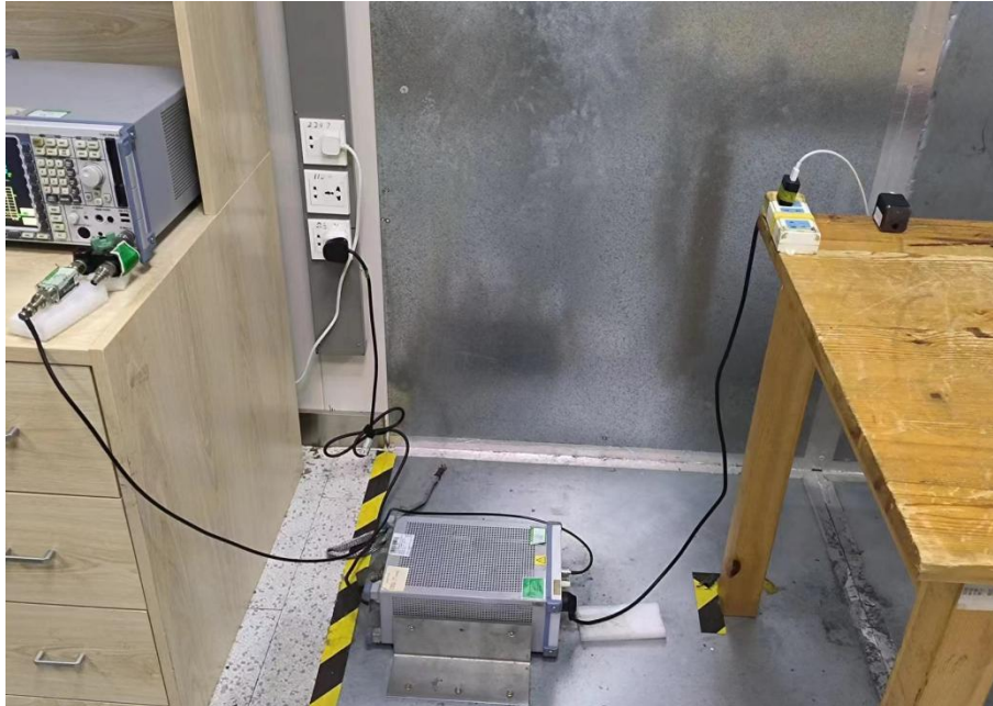
Radiated Spurious Emissions From 30MHz-1000MHz
