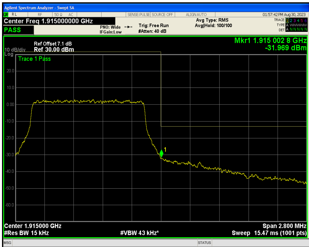
Band25 QPSK BW=3MHz Channel=26055 RB Size=15 Position=#0
