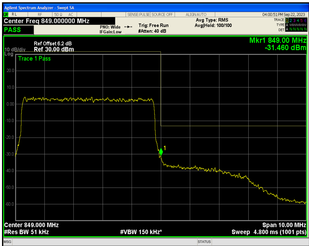
Band26(824-849) QPSK BW=10MHz Channel=26840 RB Size=50 Position=#0
