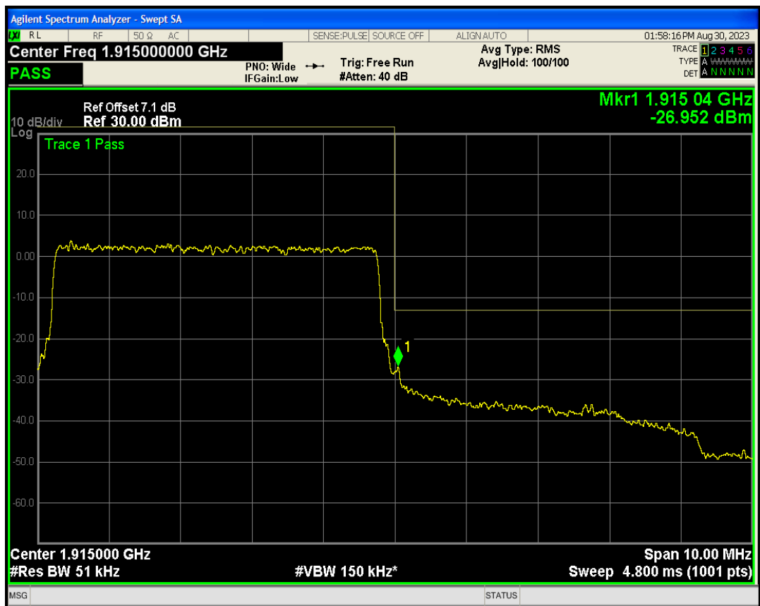
Band25 QAM16 BW=5MHz Channel=26665 RB Size=25 Position=#0
