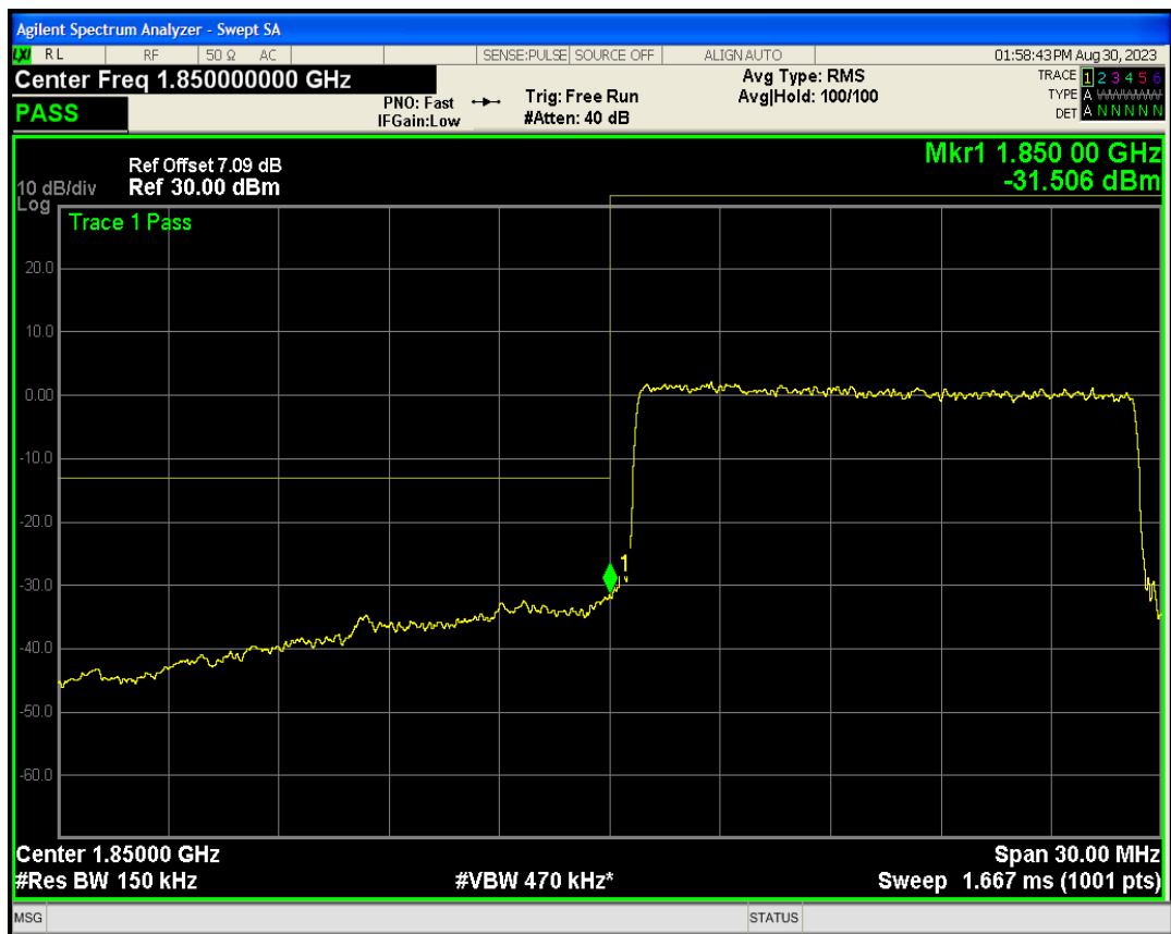
Band25 QPSK BW=15MHz Channel=26615 RB Size=75 Position=#0
