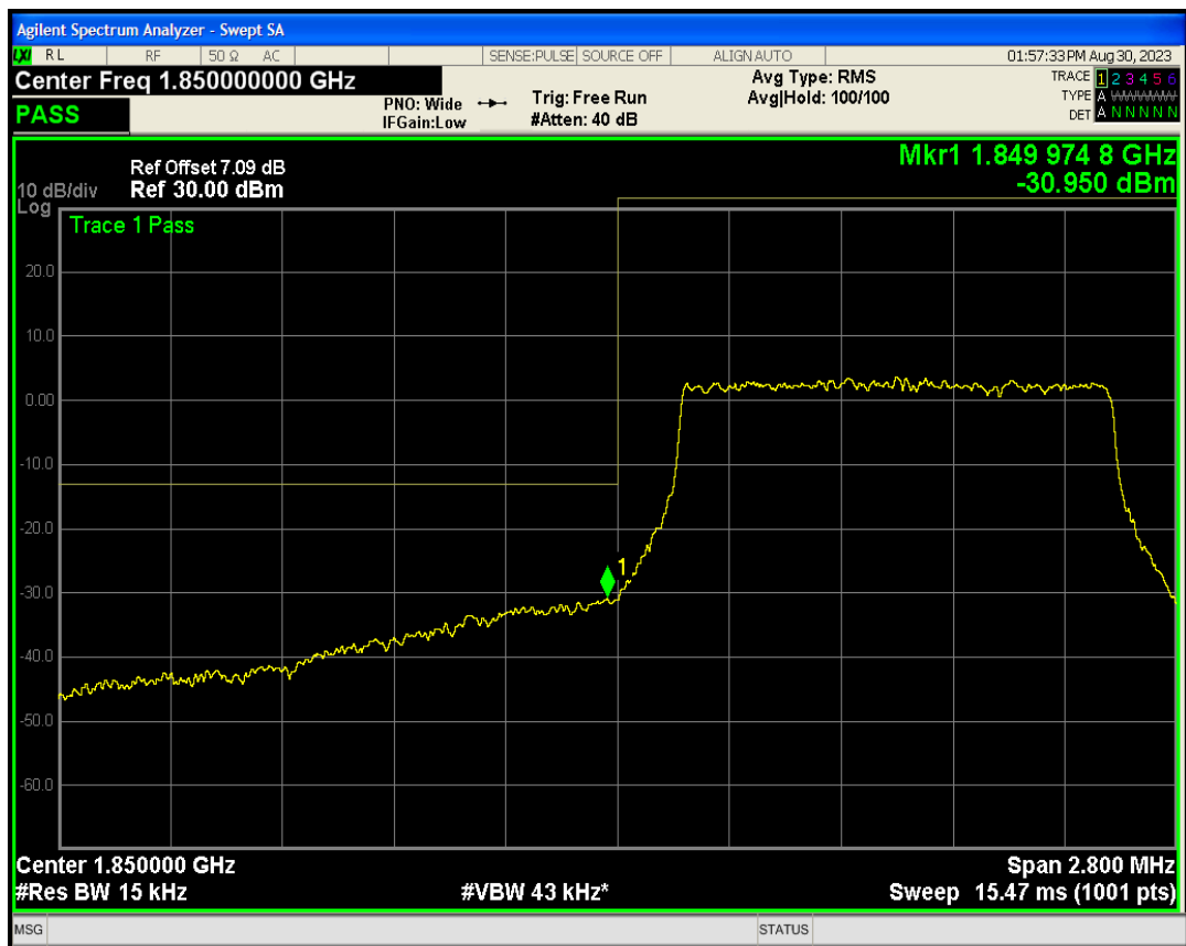
Band25 QPSK BW=1.4MHz Channel=26683 RB Size=6 Position=#0
