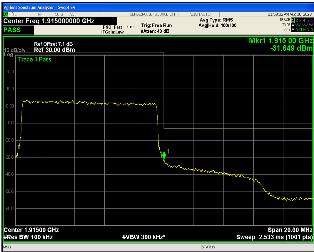
Band25 QAM16 BW=10MHz Channel=26640 RB Size=50 Position=#0
