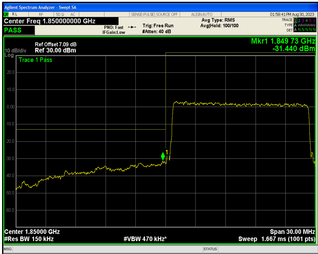
Band25 QAM16 BW=15MHz Channel=26115 RB Size=75 Position=#0
