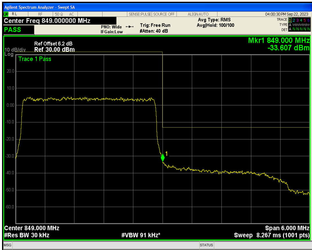
Band26(824-849) QAM16 BW=3MHz Channel=27025 RB Size=15 Position=#0
