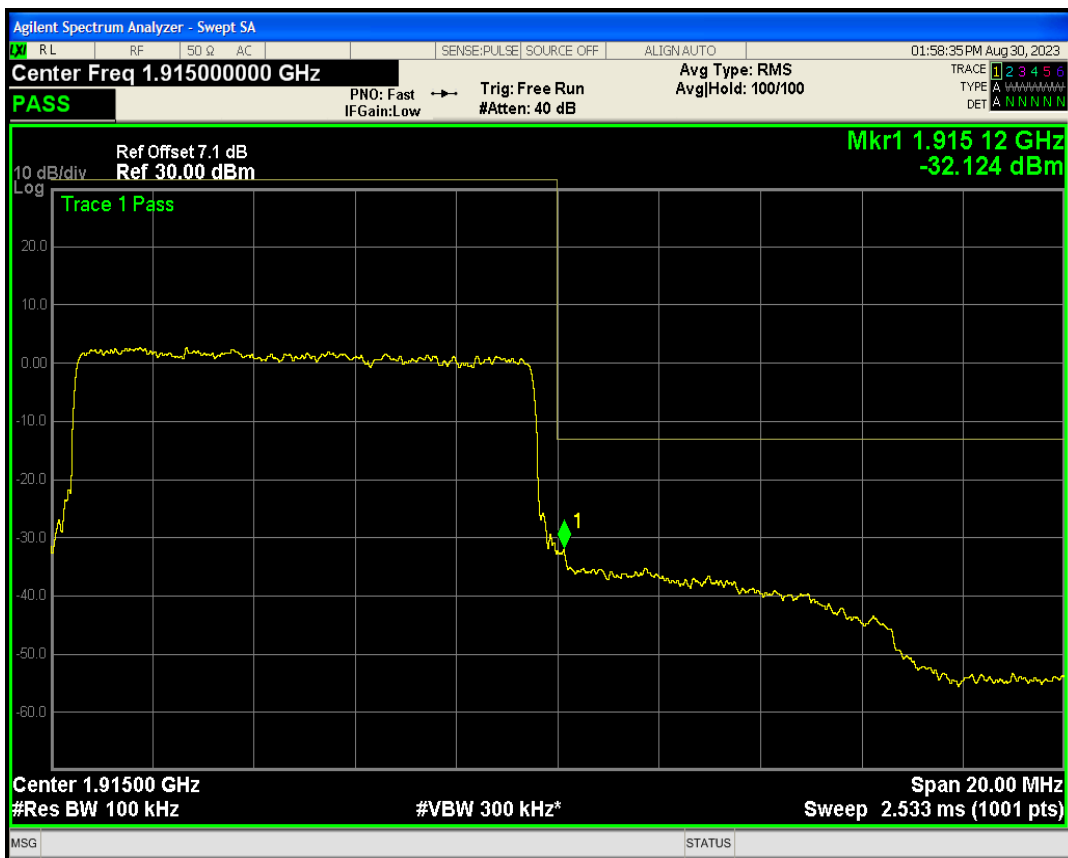
Band25 QPSK BW=15MHz Channel=26115 RB Size=75 Position=#0
