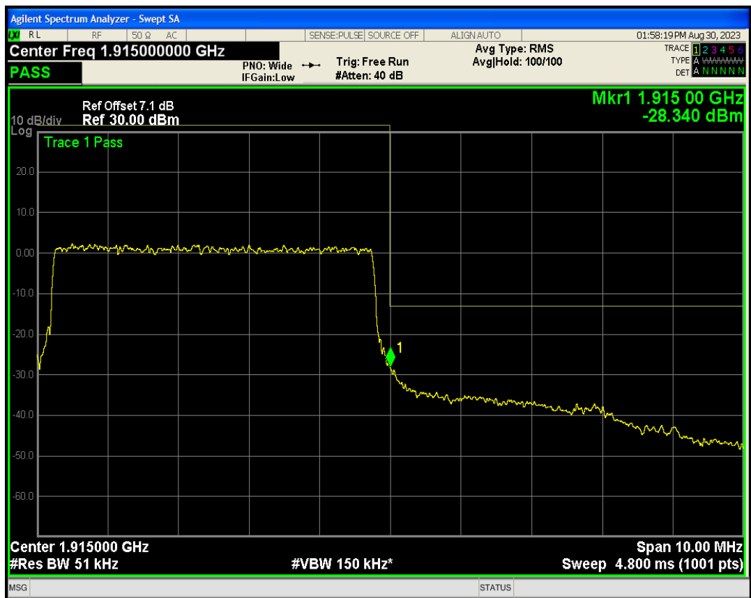
Band25 QPSK BW=10MHz Channel=26090 RB Size=50 Position=#0
