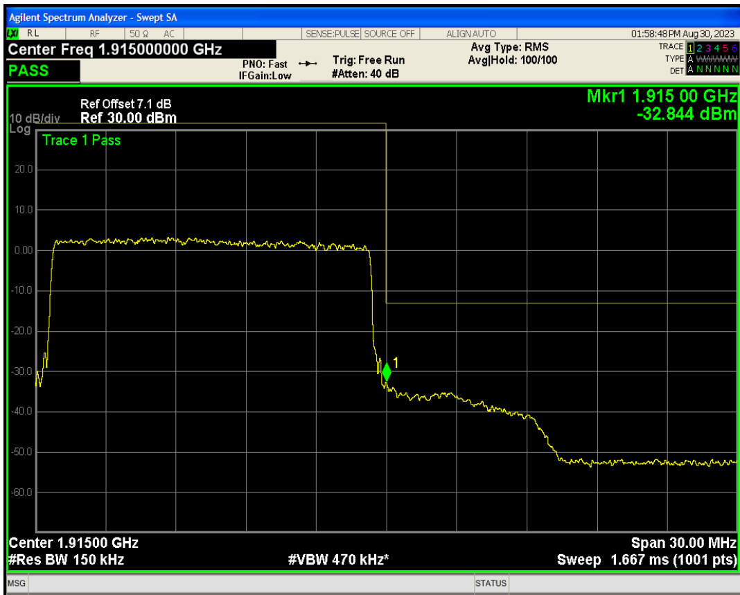
Band25 QAM16 BW=15MHz Channel=26615 RB Size=75 Position=#0
