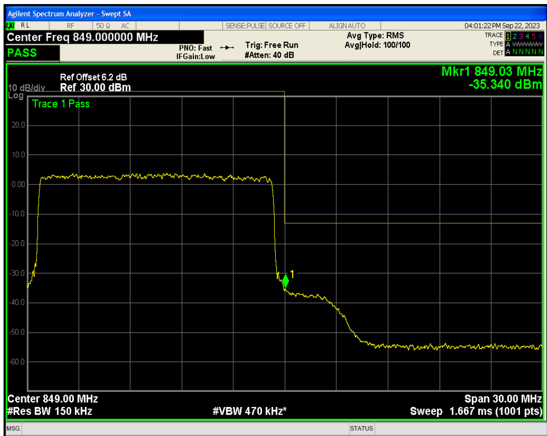
Band4 QPSK BW=1.4MHz Channel=19957 RB Size=6 Position=#0
