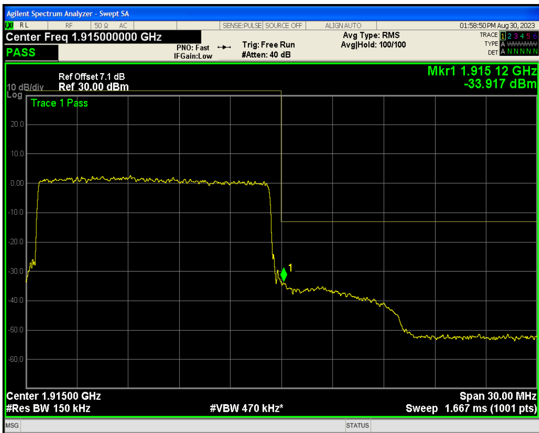
Band25 QPSK BW=20MHz Channel=26140 RB Size=100 Position=#0
