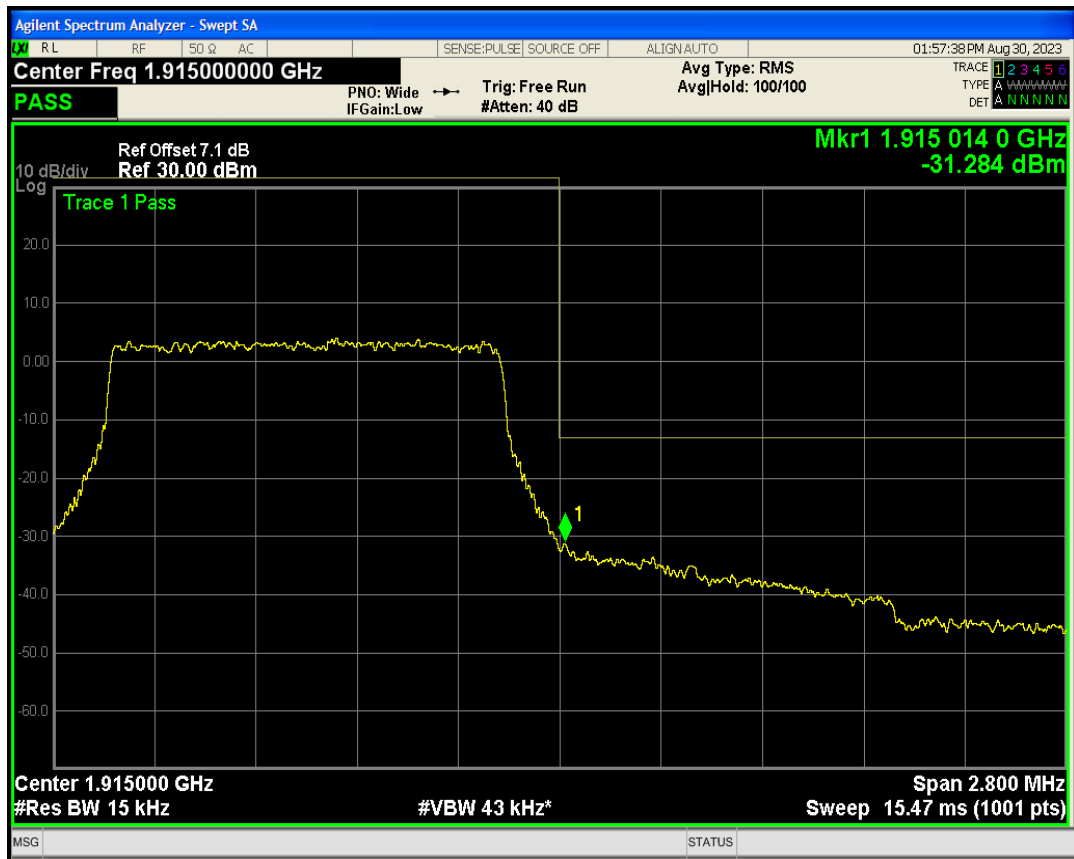
Band25 QAM16 BW=1.4MHz Channel=26683 RB Size=6 Position=#0
