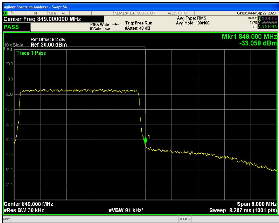
Band26(824-849) QPSK BW=5MHz Channel=26815 RB Size=25 Position=#0
