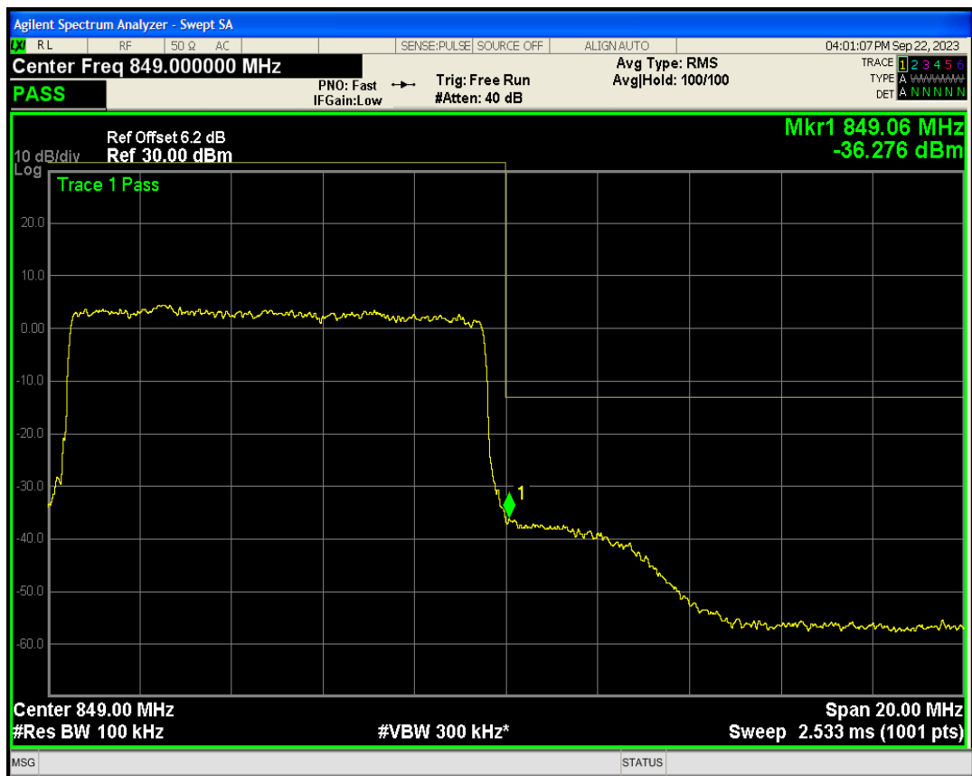
Band26(824-849) QPSK BW=15MHz Channel=26865 RB Size=75 Position=#0
