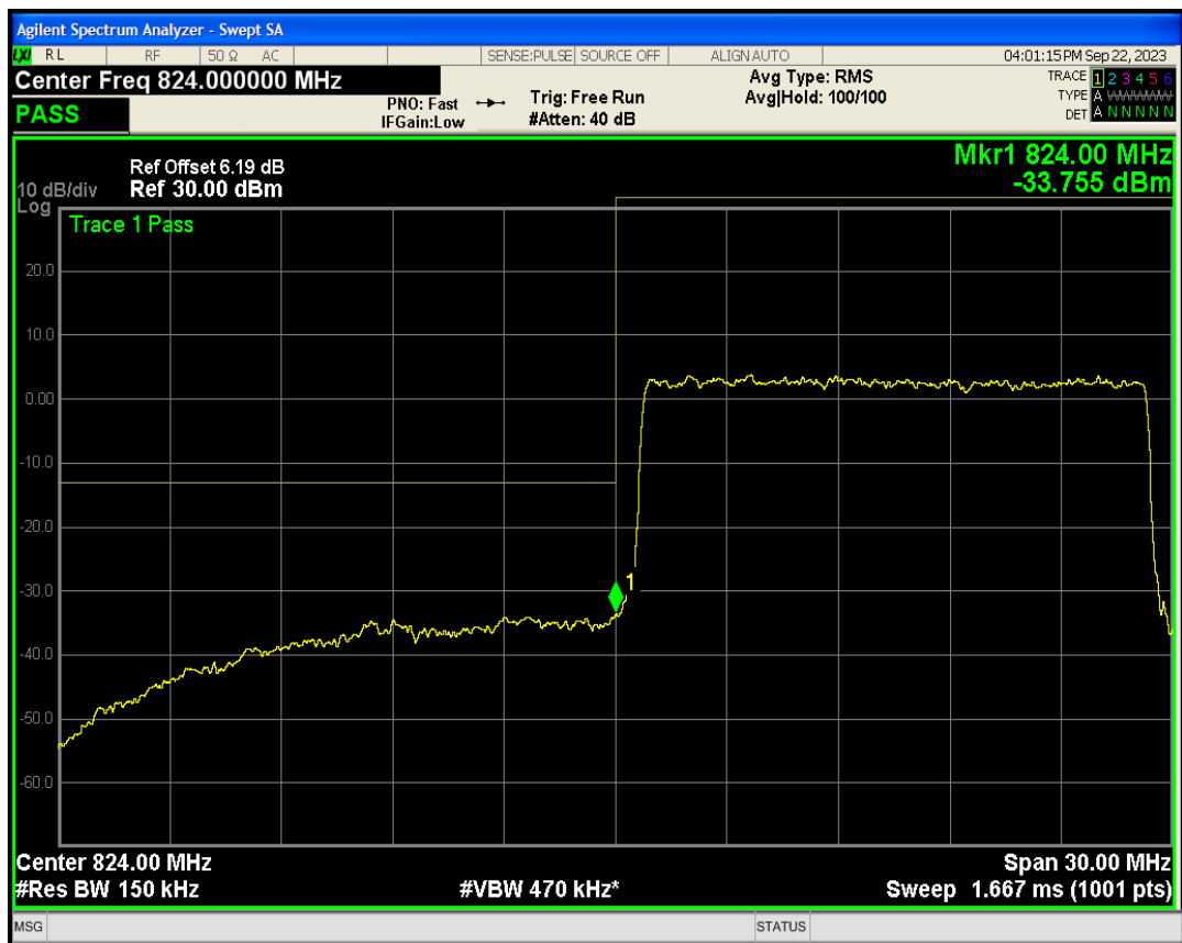
Band26(824-849) QPSK BW=15MHz Channel=26965 RB Size=75 Position=#0
