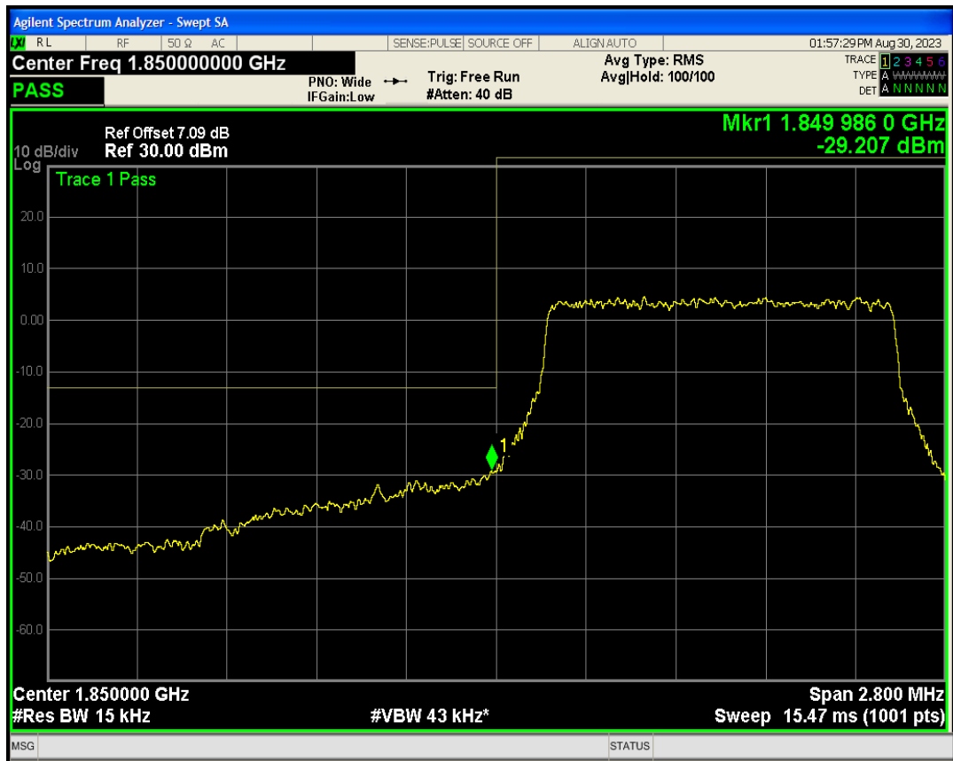
Band25 QAM16 BW=1.4MHz Channel=26047 RB Size=6 Position=#0
