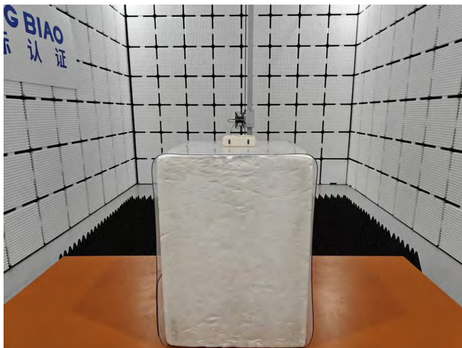
Radiated Emission Above 1GHz
