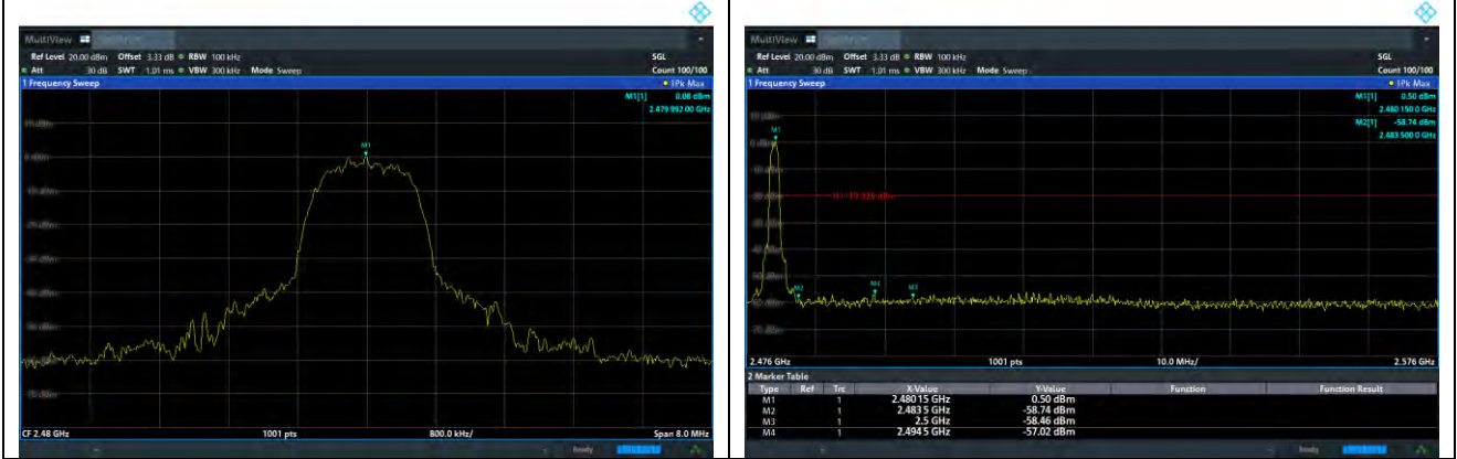
\pi/4 -DQPSK: Band Edge, Right Side
