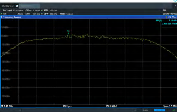
\pi/4 -DQPSK on Channel 78
