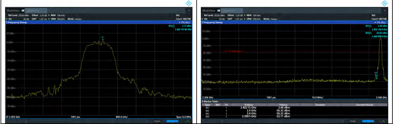
\pi/4 -DQPSK: Band Edge, Right Side
