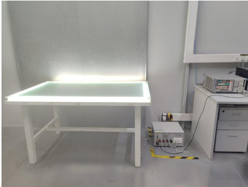
Photos of radiated emission test 30MHz – 1GHz
