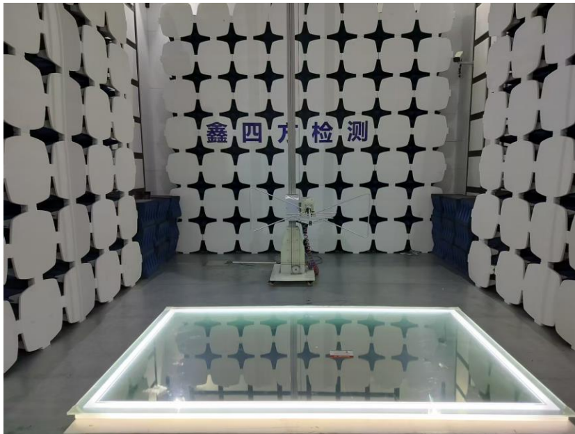
Photos of radiated emission test 30MHz – 1GHz
