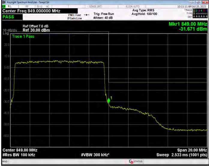
Band26(824-849) QPSK BW=10MHz Channel=26990 RB Size=50 Position=#0
