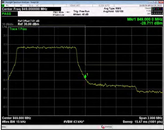
Band26(824-849) QPSK BW=10MHz Channel=26840 RB Size=50 Position=#0
