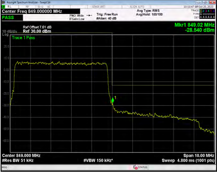
Band26(824-849) QPSK BW=5MHz Channel=27015 RB Size=25 Position=#0
