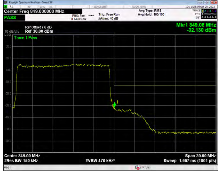
Band26(824-849) 16QAM BW=3MHz Channel=26805 RB Size=15 Position=#0
