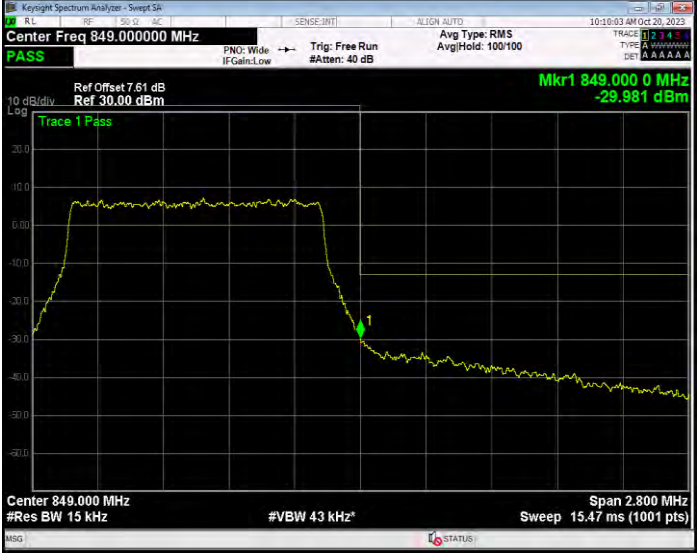
Band26(824-849) 16QAM BW=1.4MHz Channel=27033 RB Size=6 Position=#0
