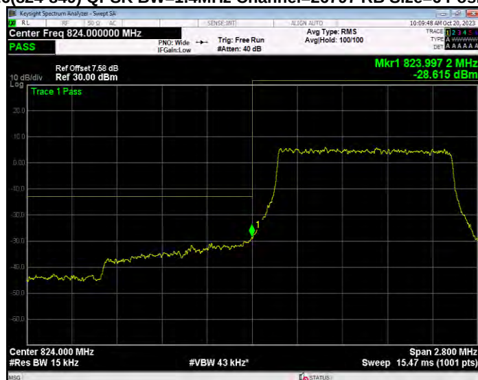
Band26(824-849) QPSK BW=1.4MHz Channel=26797 RB Size=6 Position=#0
