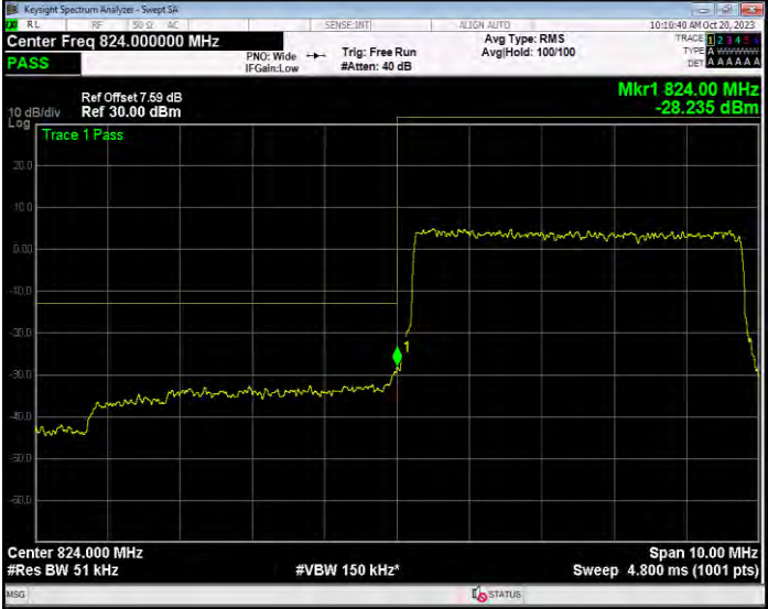
Band26(824-849) QPSK BW=5MHz Channel=27015 RB Size=25 Position=#0
