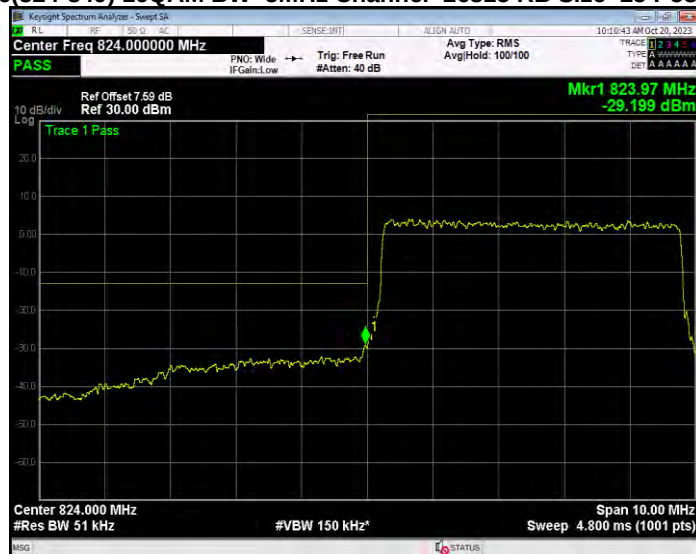
Band26(824-849) 16QAM BW=5MHz Channel=27015 RB Size=25 Position=#0
