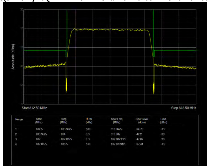
Band26(814-824) 16QAM BW=3MHz Channel=26705 RB Size=15 Position=#0
