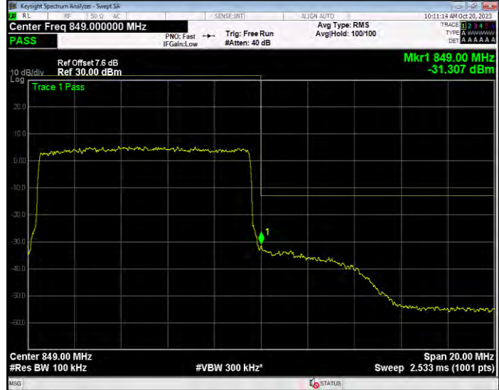
Band26(824-849) 16QAM BW=15MHz Channel=26865 RB Size=75 Position=#0
