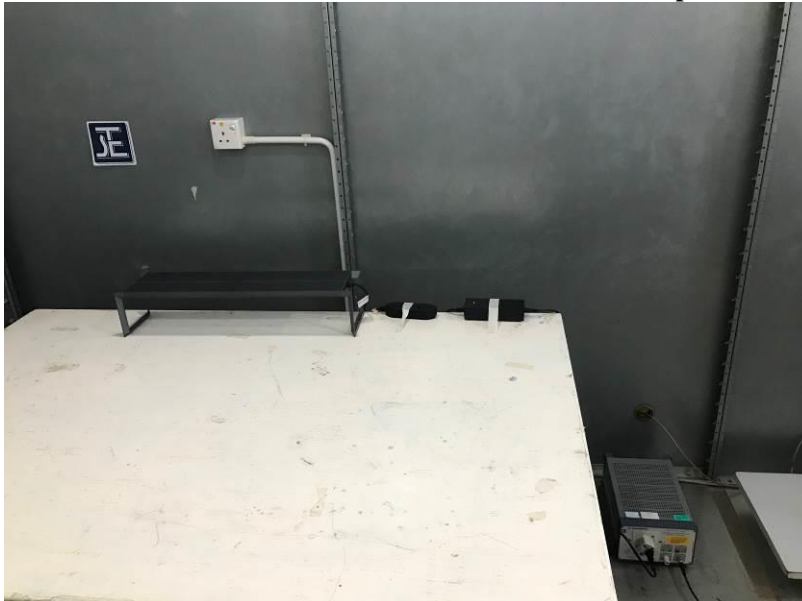
Measurement of Conducted Emission Test Set Up
