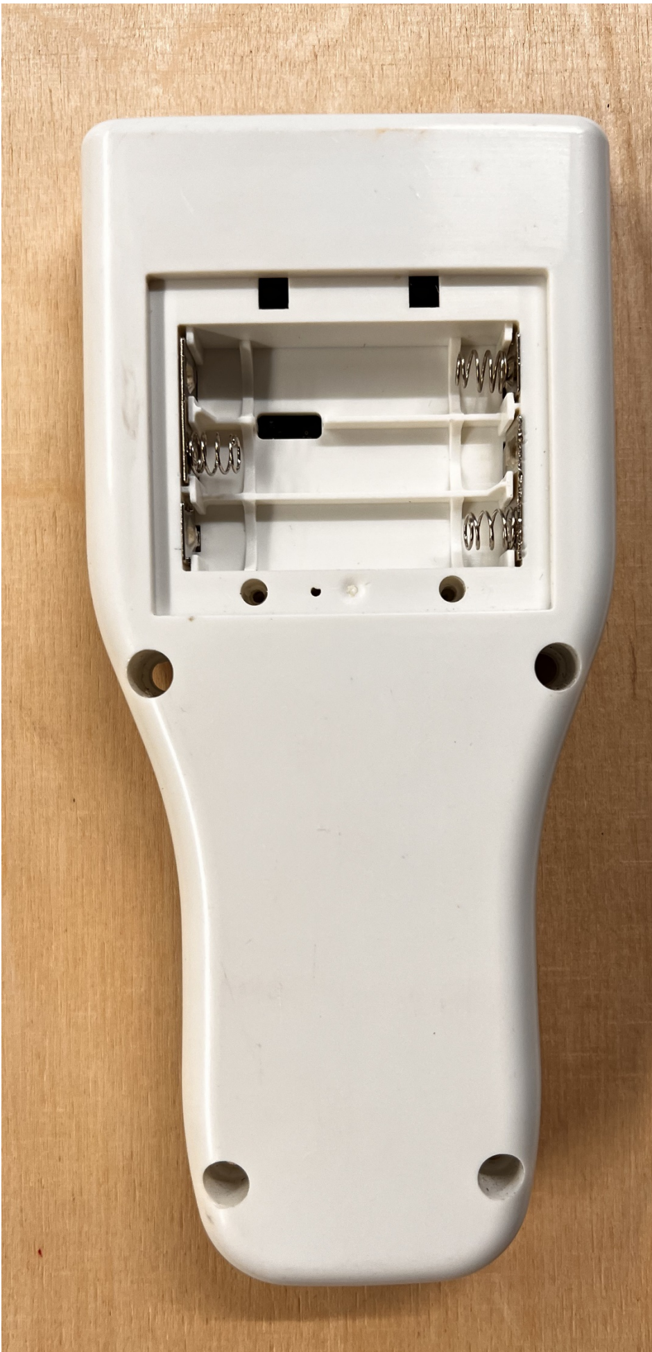
Back of Device with Cover and Batteries Removed
