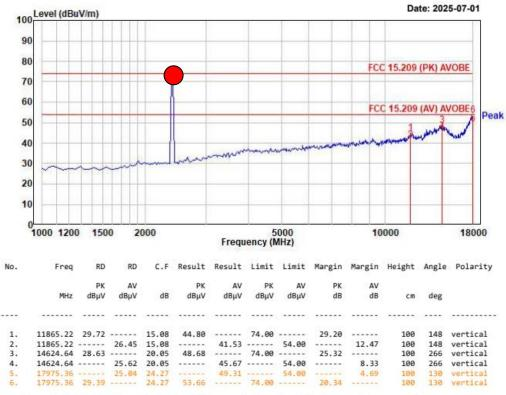
Remarks: C.F (Correction Factor) = Antenna factor + Cable loss - Preamp gain
