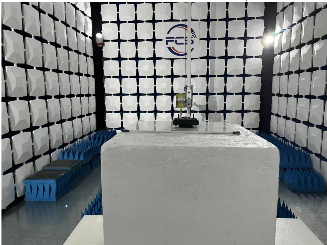
Above 1GHz for radiated emission test setup
