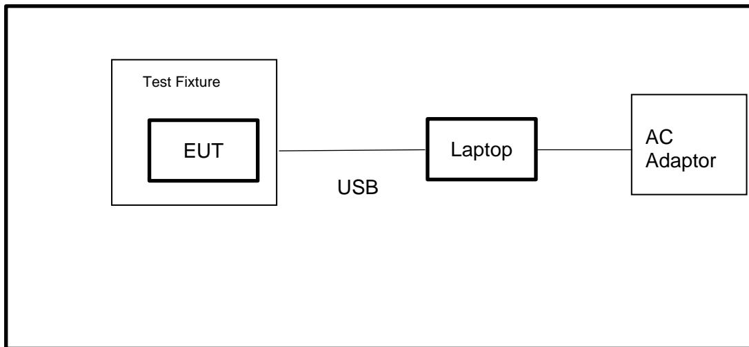
Note: AC Adaptor only use for AC POWER LINE CONDUCTED EMISSION test.
