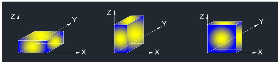
Note 1: For all radiated test, EUT in each of three orthogonal axis emissions had been tested, but only the worst case (X axis) data recorded in the report.
