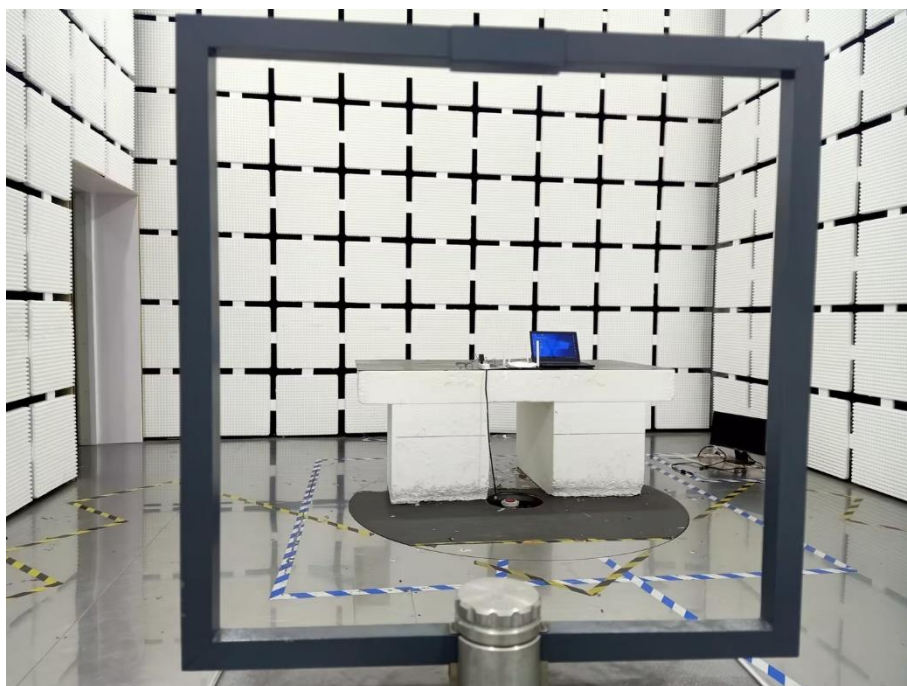
Radiation Emission Test Setup (Below 30MHz)
