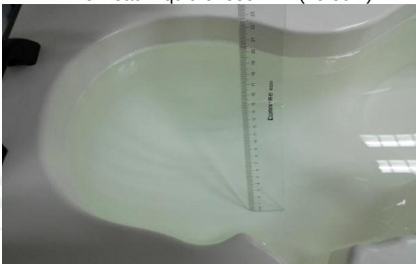
The Head Liquid of 2600MHz (15.1cm)
