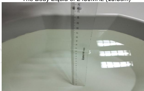
The Body Liquid of 5000-6000MHz (16.5cm)
