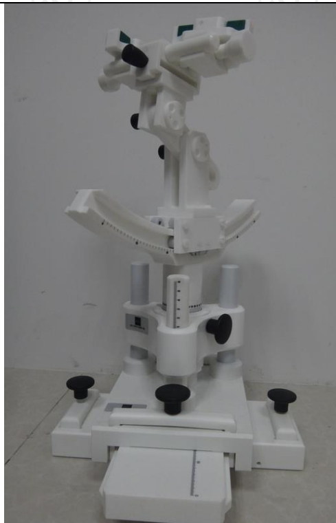
COMOSAR Mobile phone positioning system
