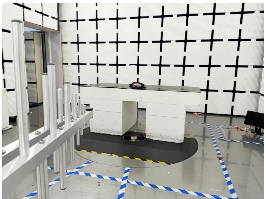
Radiation Emission Test Setup (30MHz to 1GHz)
