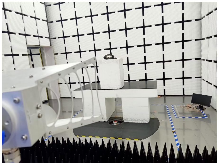
Radiation Emission Test Setup (1GHz to 18GHz)
