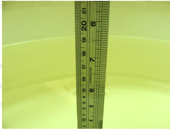
Photo of Liquid Height for Body SAR
