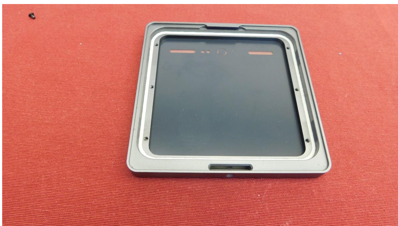
Picture 8: Housing without keyboard layout internal view
