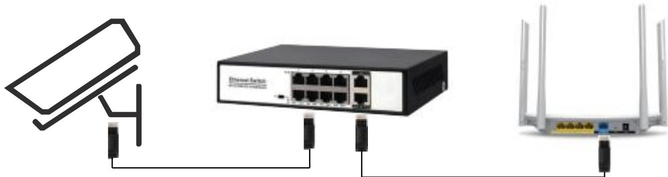
3. Install the camera to outside, POE Switch support 100meters(CAT5) max.
