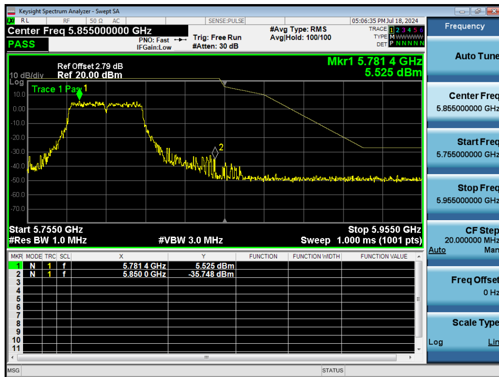
Band Edge NVNT ac40 5795MHz High Ant1
