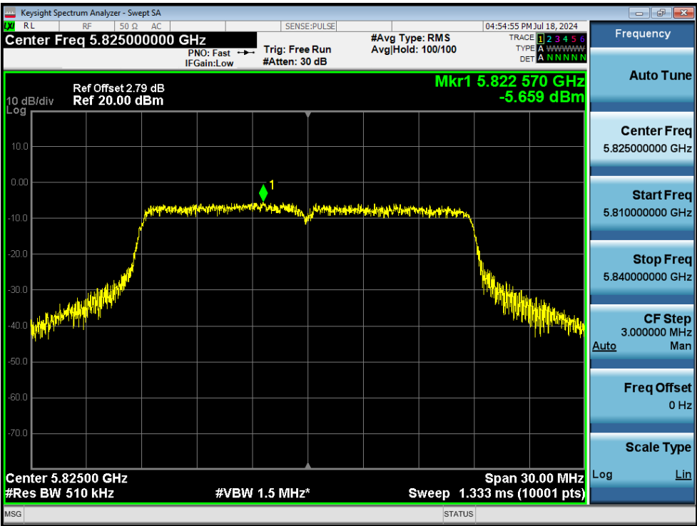
PSD NVNT n20 5825MHz Ant1
