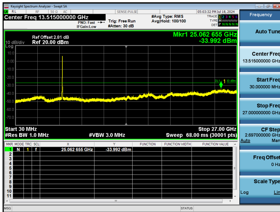
Tx. Spurious NVNT ac40 5755MHz Ant1 Emission
