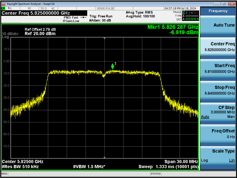
PSD NVNT ac20 5825MHz Ant1
