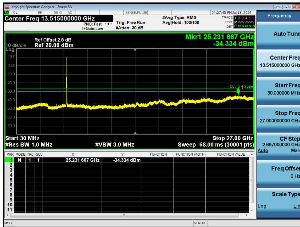
Tx. Spurious NVNT n20 5745MHz Ant1 Emission
