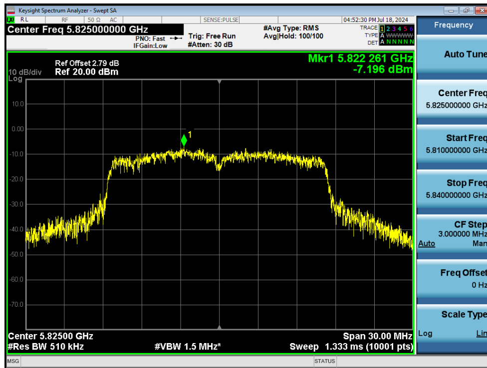
PSD NVNT a 5825MHz Ant1
