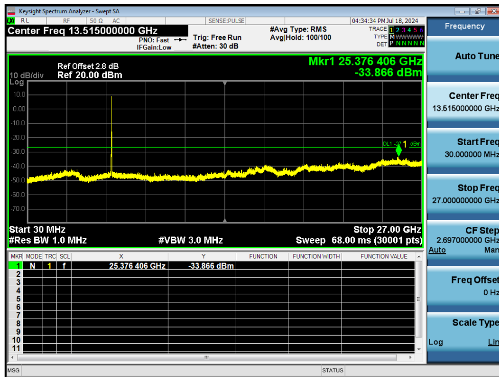
Tx. Spurious NVNT ac20 5785MHz Ant1 Emission
