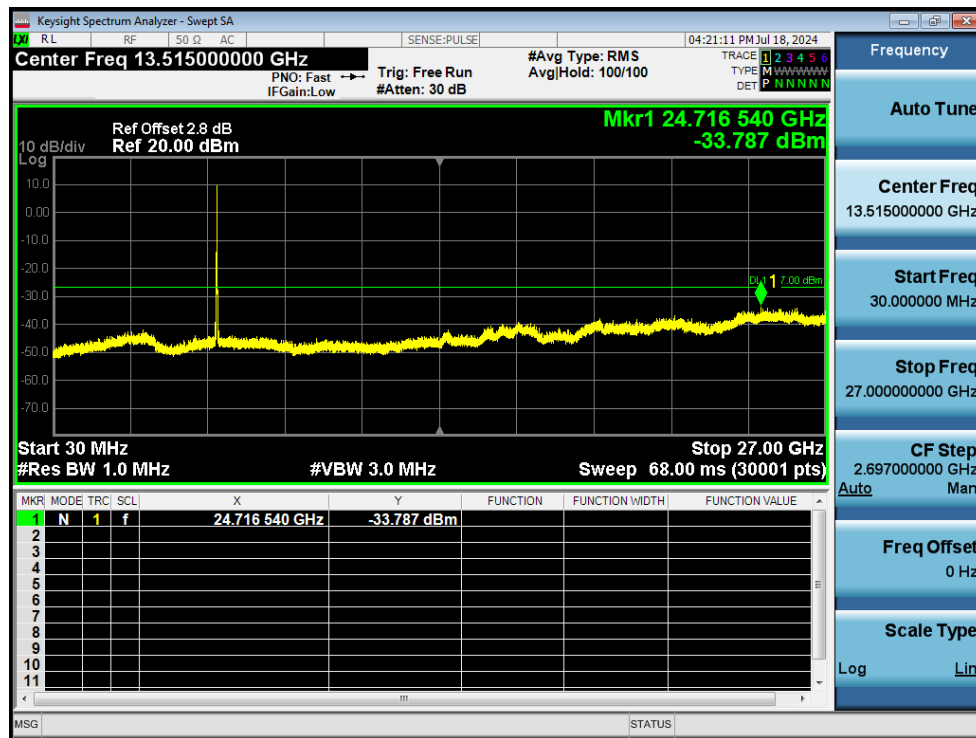
Tx. Spurious NVNT a 5745MHz Ant1 Emission
