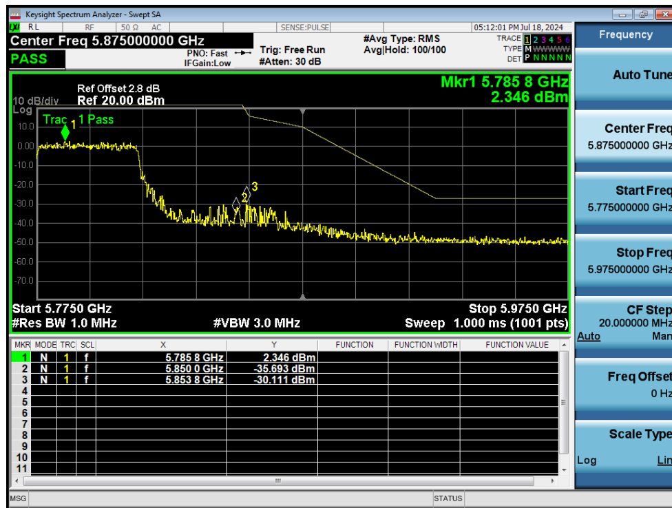
Band Edge NVNT ac80 5775MHz High Ant1
