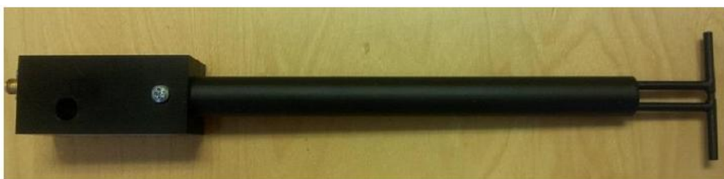
Figure 1 – MVG COMOSAR Validation Dipole
