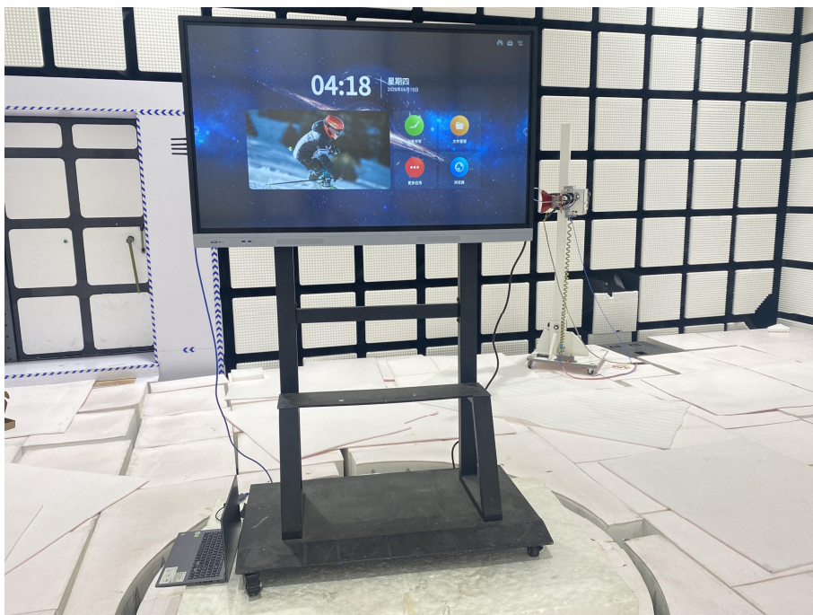
Radiated spurious emission Test Setup-2(Above 1GHz)
