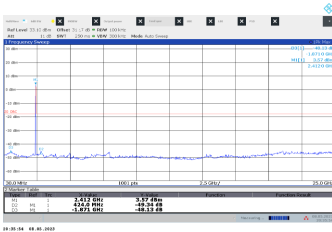
Figure 7.6-3: Conducted spurious emissions on low channel
