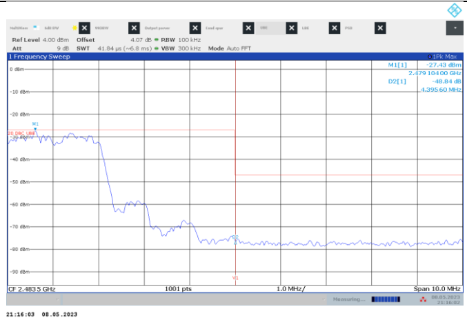
Figure 7.6-2: Band edge spurious emissions at high band edge
