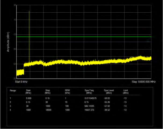
Band4 QPSK BW=1.4MHz Channel=20175 RB Size=1 Position=#0
