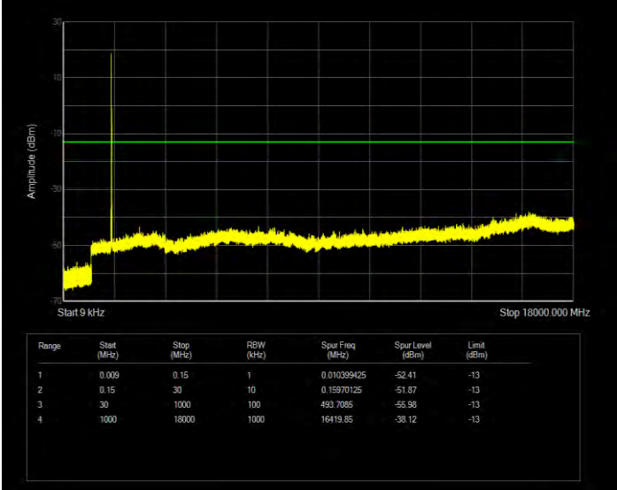
Band4 QPSK BW=10MHz Channel=20000 RB Size=1 Position=#0
