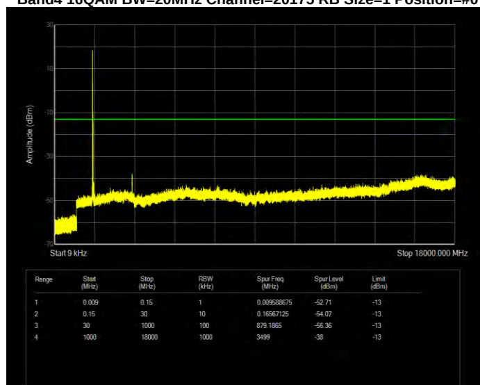
Band4 16QAM BW=20MHz Channel=20175 RB Size=1 Position=#0
