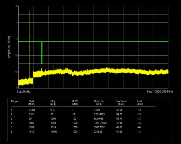
Band13 QPSK BW=10MHz Channel=23230 RB Size=1 Position=#0
