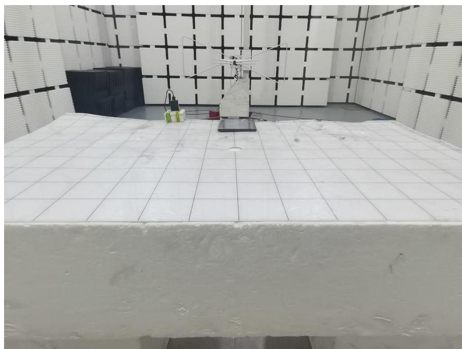
**Set-up for Radiated Emission (RE), Above 1GHz**
