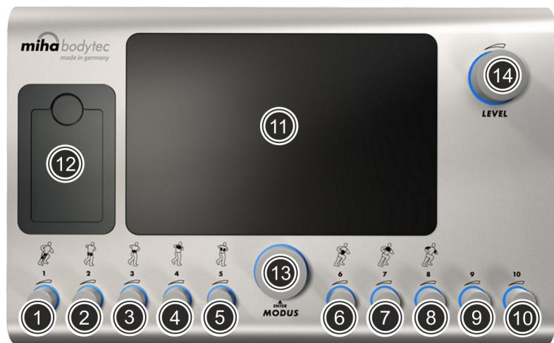
Fig. 3: Control unit (top side)
