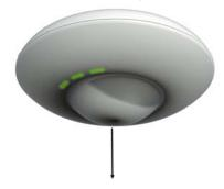
Record the location and ID number of the base station during installation, so that the anchor coordinates can be set when the system is debugged.
