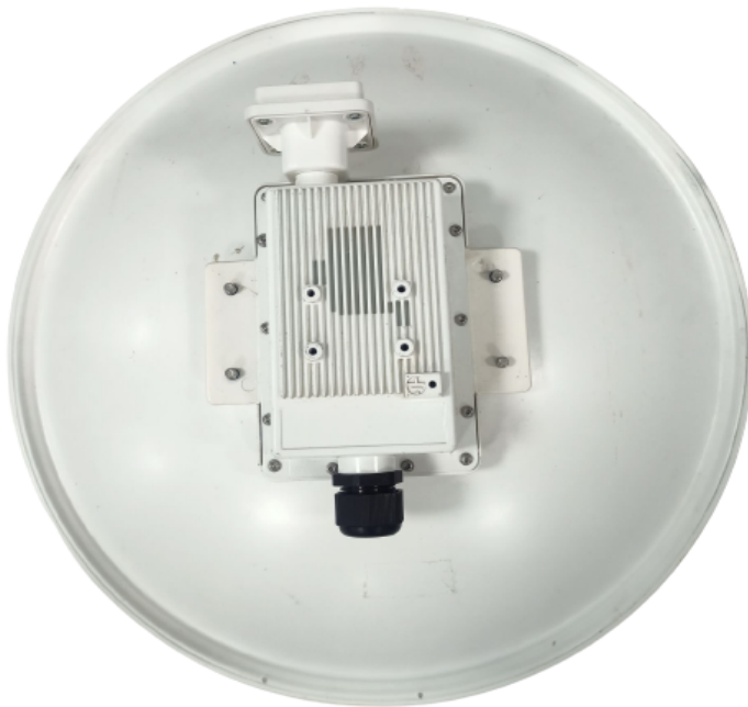
Figure 4: Back view of the 2x2 UBR(UBAX) with 25dB S Dish Antenna
