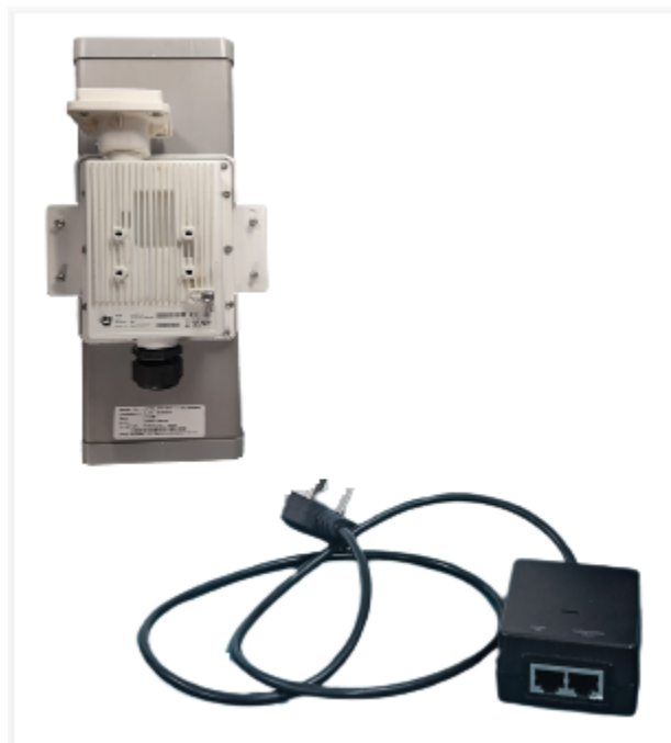
Figure 9: Basic overview of the device UBR (UBAX) power up with 25dB Dish Antenna
