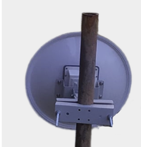
Figure 13: Basic overview of pole mounted 2x2 UBR (UBAX) device
