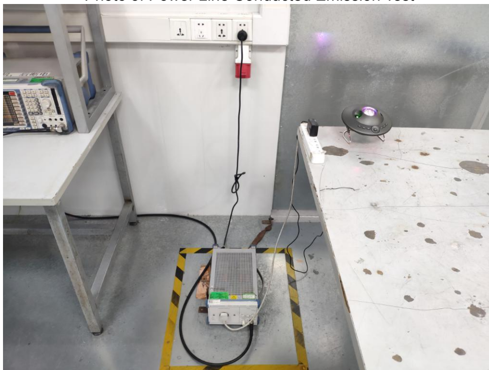
Photo of Power Line Conducted Emission Test
