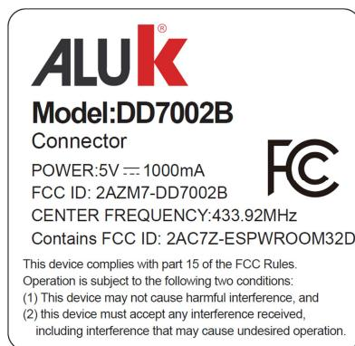
Specifications: The label shall be securely affixed to a permanently attached part of the device, in a location where it is visible or easily accessible to the user, and shall not be readily detachable. The label shall be sufficiently durable to remain fully legible and intact on the device in all normal conditions of use throughout the device's expected lifetime.
