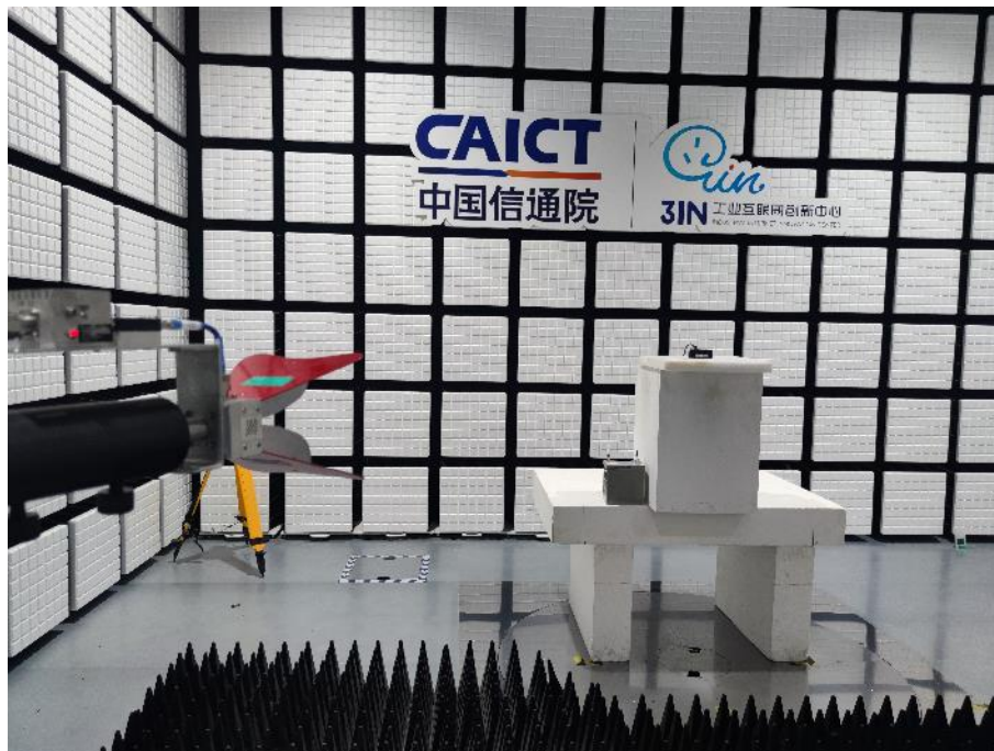
Description: Radiated Emission Test Setup (1 GHz -18GHz)
