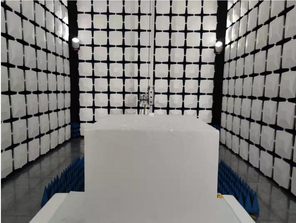
Above 1GHz for radiated emission test setup
