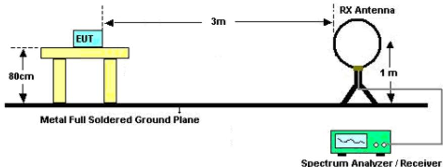
For radiated emissions from 30MHz to 1GHz
