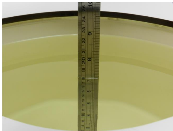
Fig 11.1 Photo of Liquid Height for Body SAR
