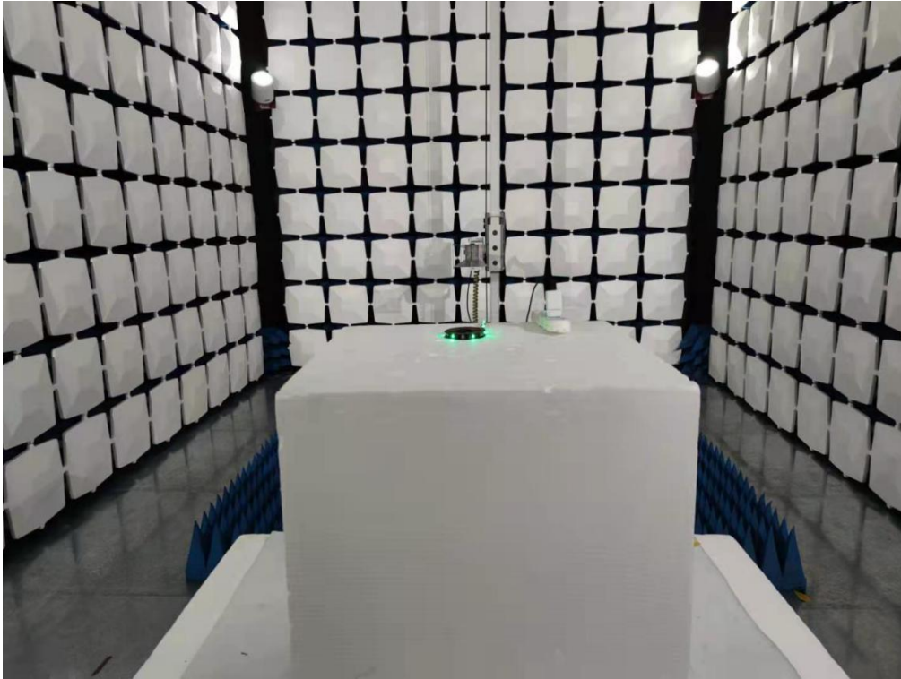
Above 1GHz for radiated emission test setup
