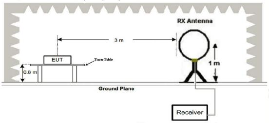
2. Radiated Emission Test-Up Frequency 30MHz~1GHz
