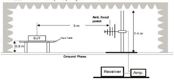
3. Radiated Emission Test-Up Frequency Above 1GHz
