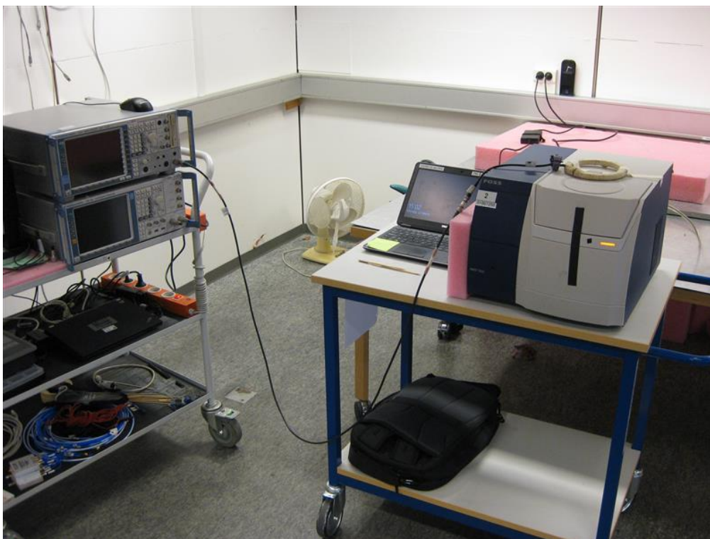
Photo 4.5.1 Test setup regarding measurement of 20 dB bandwidth/occupied BW.
