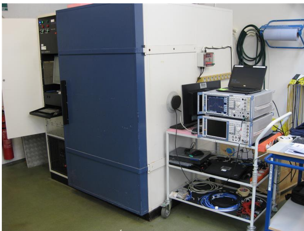
Photo 4.8.2 Test setup regarding measurement of Frequency stability.
