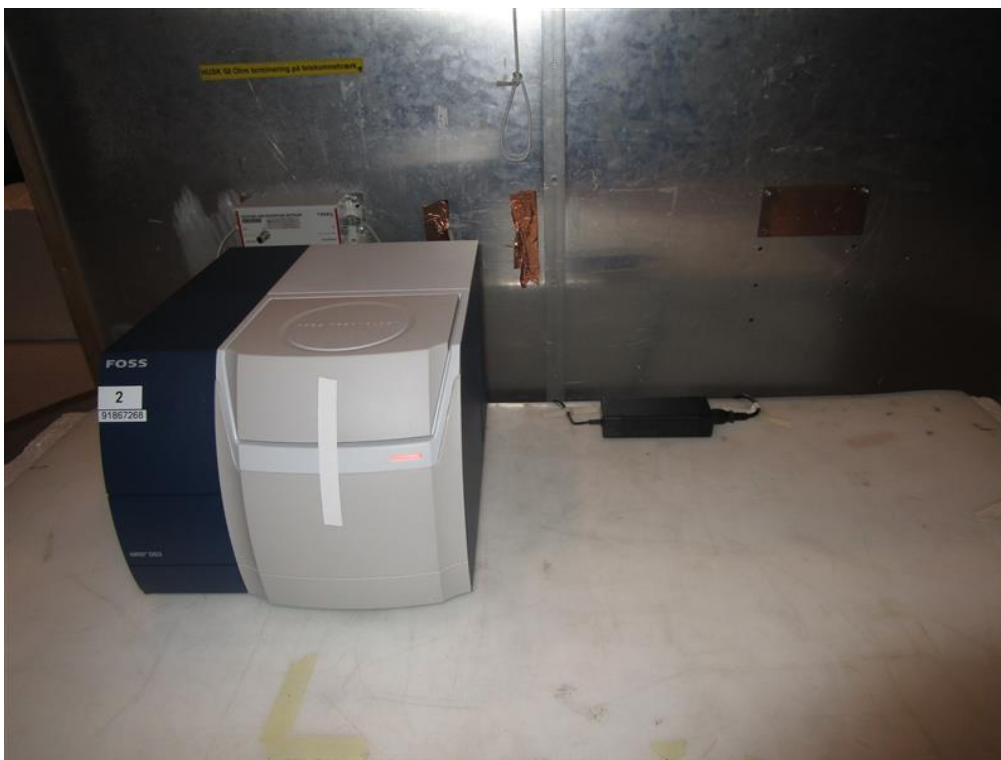
Photo 4.1.1 Test setup regarding measurement of radio frequency voltage on mains/ conducted limits.
