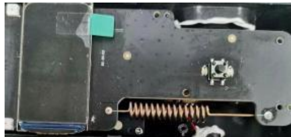
Antenna position and placement method
