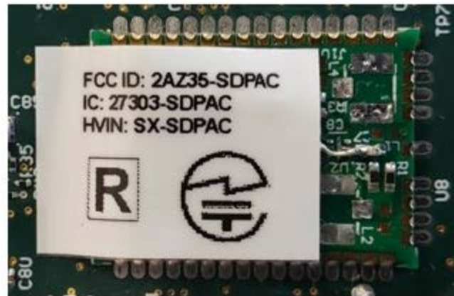
New Label placed over existing label.
