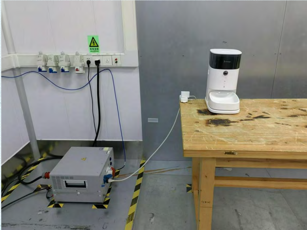
Conducted Emission at AC power line
