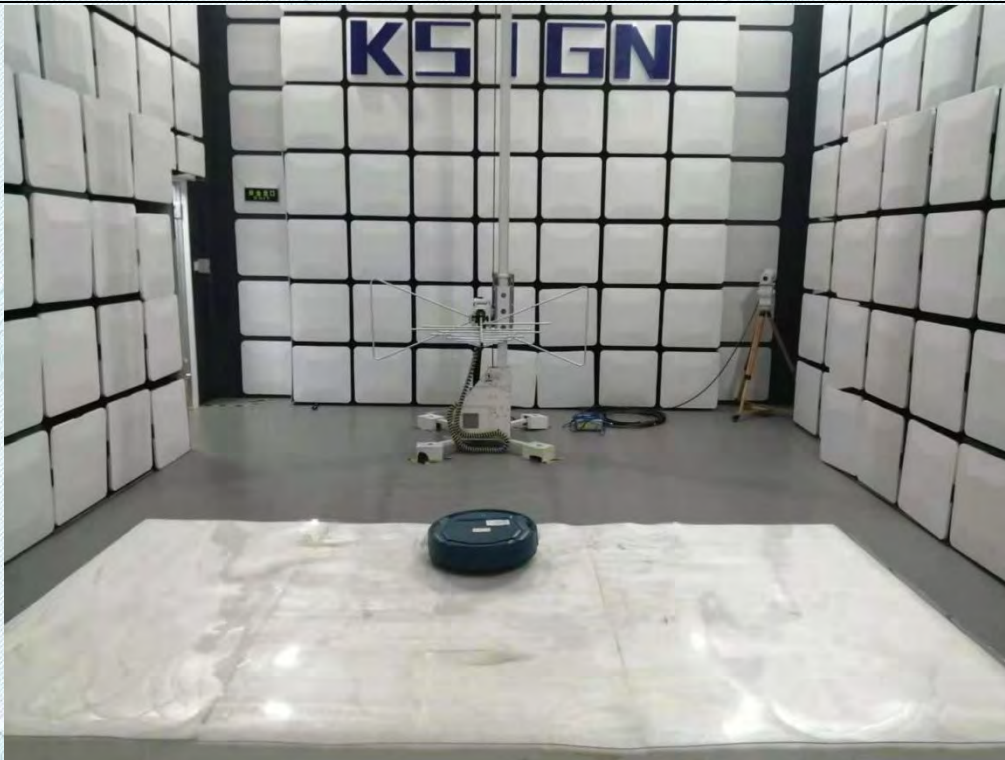
Emissions in restricted frequency bands (below 1GHz)
