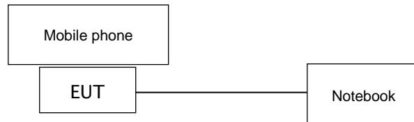
This example is connection diagram of EUT test configurations.
