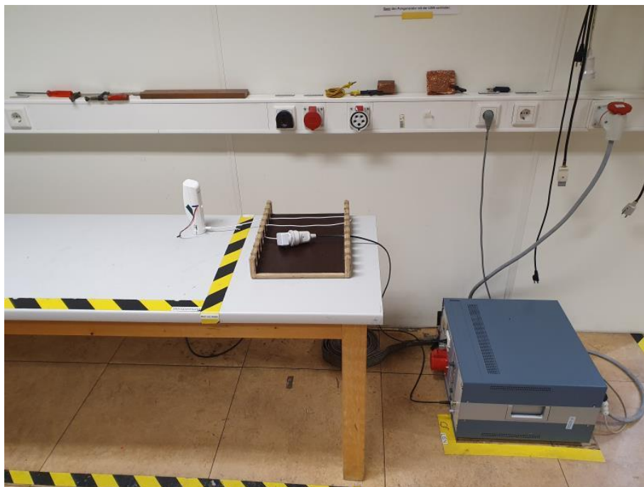
Test Setup: Conducted Emission Measurements
