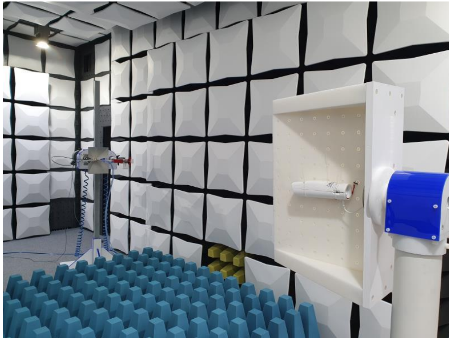
Test Setup: Radiated Measurements (1 GHz to 25 GHz)
