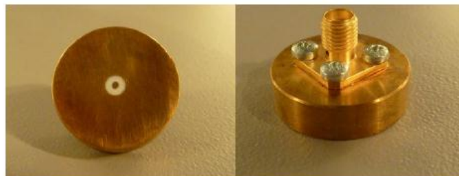
Figure 1 – MVG LIMESAR Dielectric Probe
