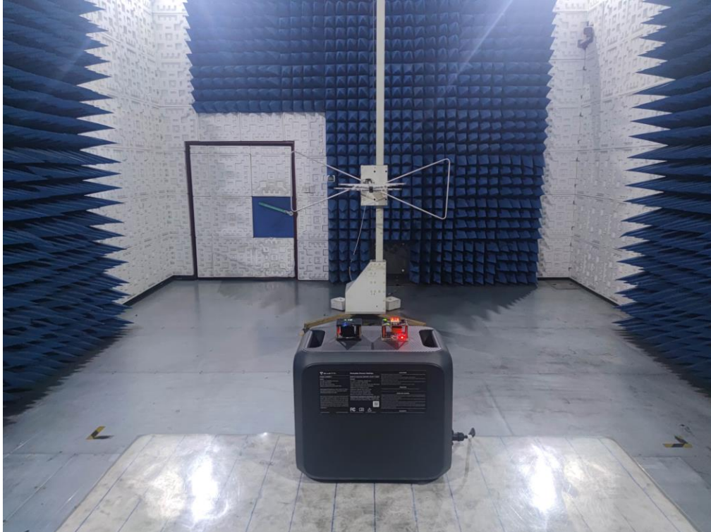
RADIATED EMISSION TEST SETUP ABOVE 1GHz
