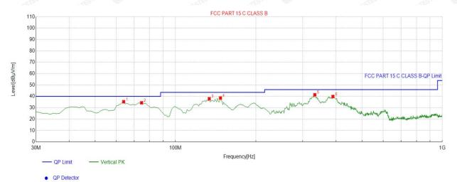
Suspected List Margin Freq. Factor Reading Level Limit Height Angle NO. **Polarity** [cm] [MHz] [dB] [dBµV/m] [dBµV/m] [dBµV/m] [dB] [°] 63.9840 -16.16 51.43 35.27 40.00 Vertical 1 4.73 100 169 74.6647 -18.51 52.87 34.36 40.00 5.64 100 66 Vertical 133.8939 -18.81 56.73 37.92 43.50 5.58 100 169 Vertical 147.4875 -19.00 57.56 38.56 43.50 4.94 100 193 4 Vertical 332.9429 -11.60 53.02 41.42 46.00 4.58 100 34 Vertical 389.2593 -10.66 50.56 39.90 46.00 6.10 100 Vertical 114
