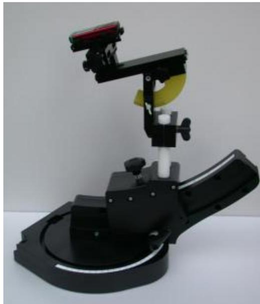
The positioning system allows obtaining cheek and tilting position with a very good accuracy. Incompliance with CENELEC, the tilt angle uncertainty is lower than  $1^\circ$ .
