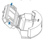
C. Take out the filter filter cotton inside the dust box, and clean it with a brush or cloth.
