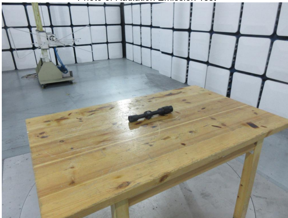
Photo of Radiation Emission Test
