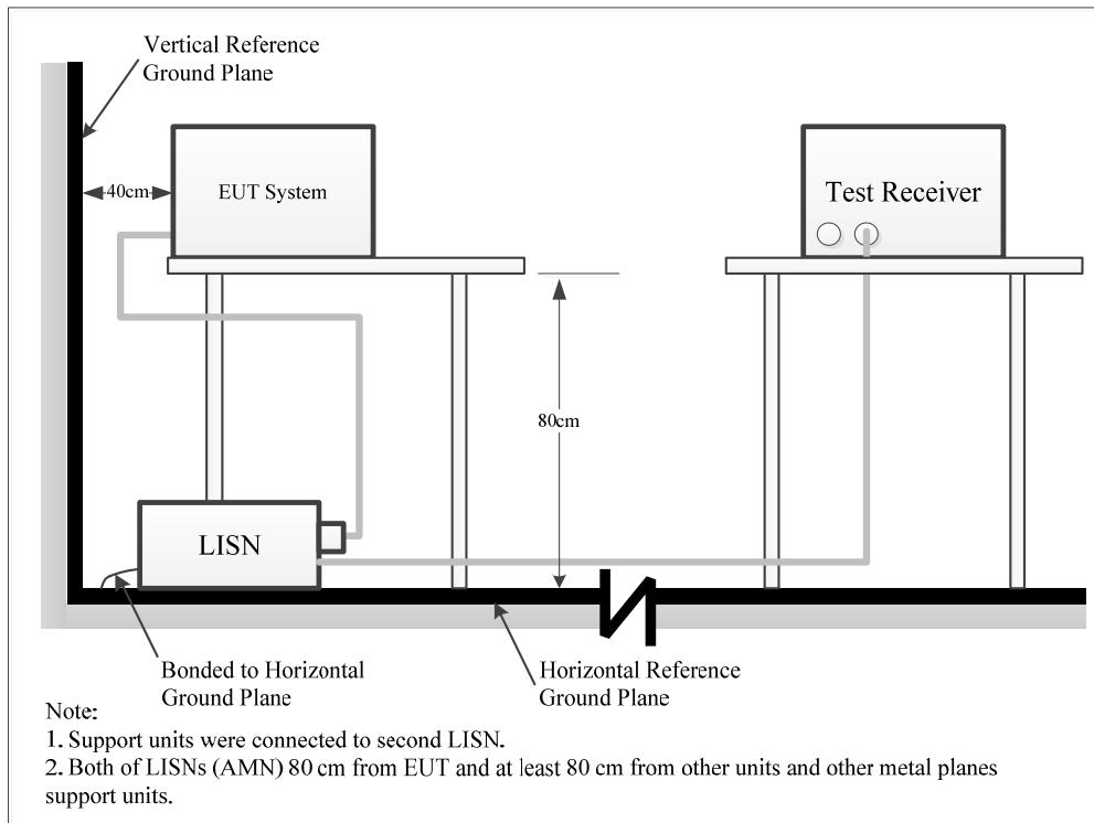
The setup of EUT is according with per ANSI C63.10-2020 measurement procedure. The specification used was with the FCC Part 15.207 limits.
