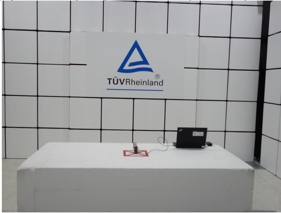
Photograph 2: Test Setup for Spurious Emissions (Front View 2)
