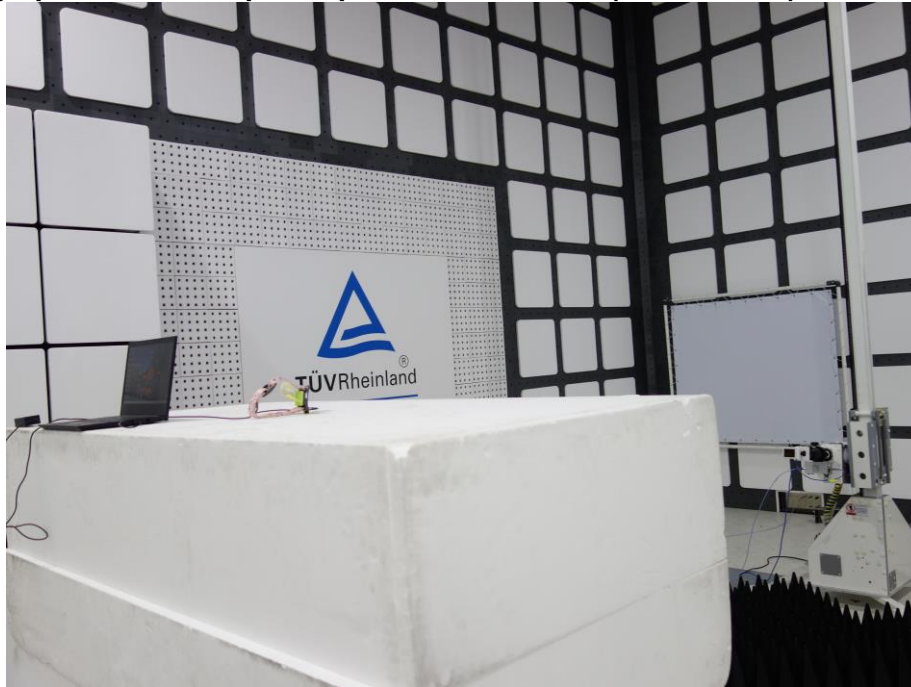
Photograph 4: Test Setup for Spurious Emissions (Back View 2)
